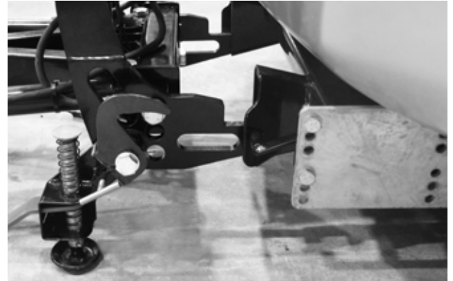
2 Align car and broom, slowly drive car forward
