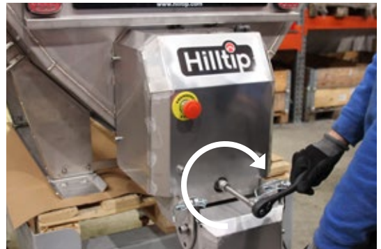
Rotate auger manually by turning it clockwise
