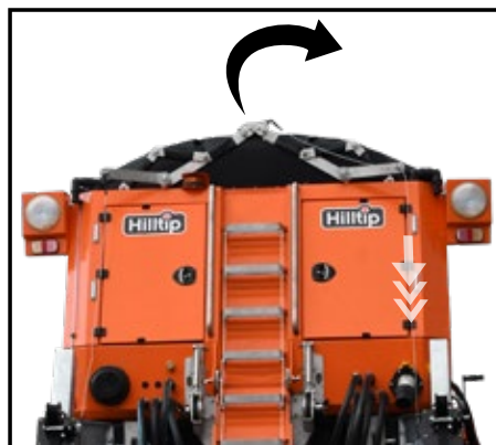
2. Pull right wire to open the right side of the tarp cover.
