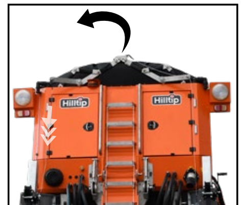
3. Pull left wire to open the left side of the tarp cover.
