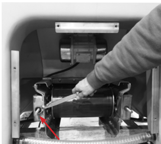
When tightening the left nut, the conveyor moves to the right and vice versa.
