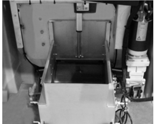
2. Spin the conveyor until you see the joint.
