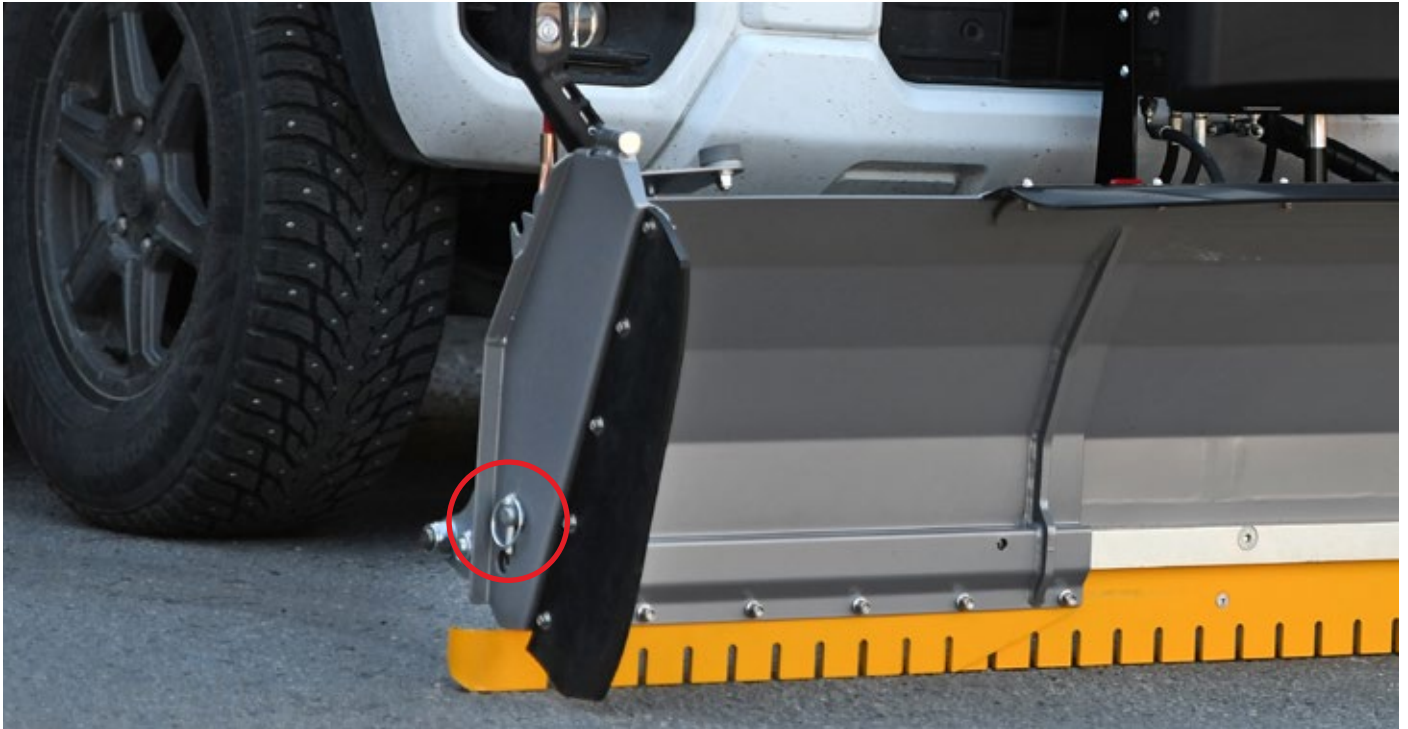
1. Pull out the linchpin on the side of the end guiding plate
