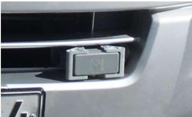
2. Fasten the connector-assembly far into the bumper to make it less visible
