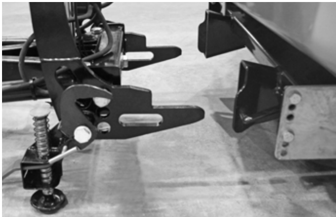
1 Plow must be standing steady on the ground, with plow shoes lowered
