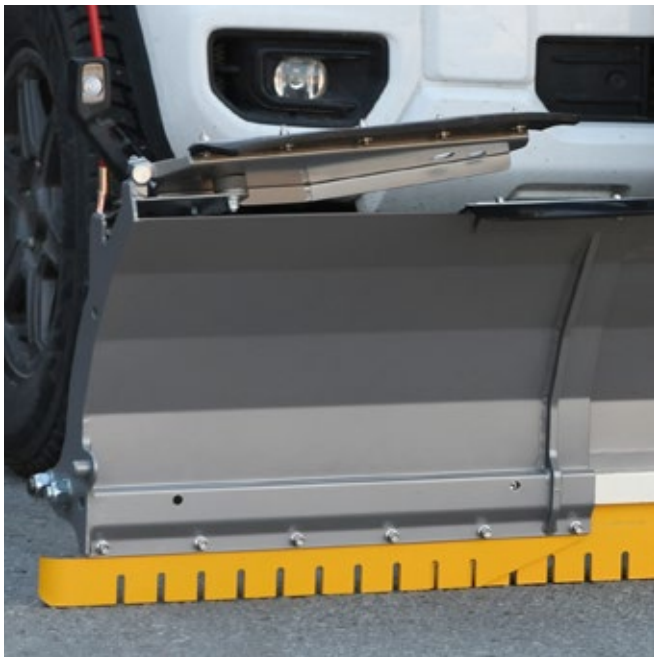
2. Manually fold up the end guiding plate
