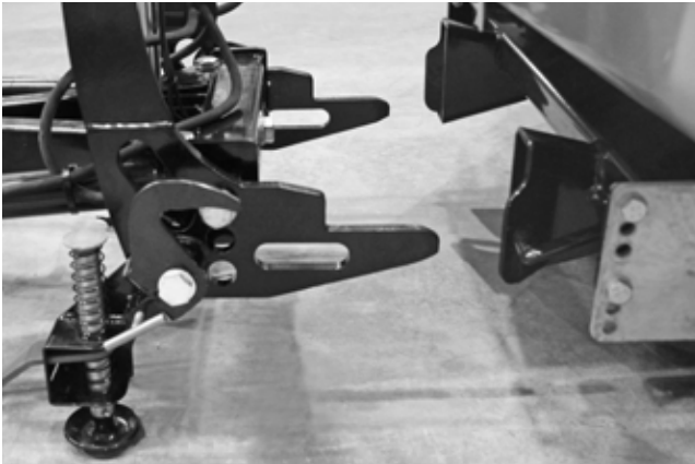
1 Plow must be standing steady on the ground, with plow shoes lowered
